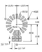
SOLDER PATTERN NOTE: Use plated thru vias (Ø0.3) under unit for heat dissipation.
